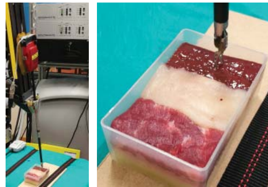
Fig. 1. Left: The bipolar forceps with integrated EBI sensor. Right: The phantom made of 3 different ex-vivo animal tissue samples, pork muscle (left), chicken breast (centre) and beef liver (right). The rough phantom dimensions are 88 \times 55 \times 25 mm.
